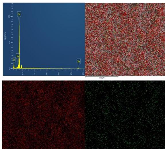
Figure 6. EDX spectrum of (a) Se sample and mapping (b) of sample, (c) Se mapping and (d) O mapping.
