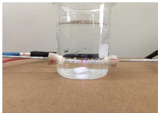
Figure 1. Synthesis process of nano selenium after 60 mins of reactions using distilled water solvent.
