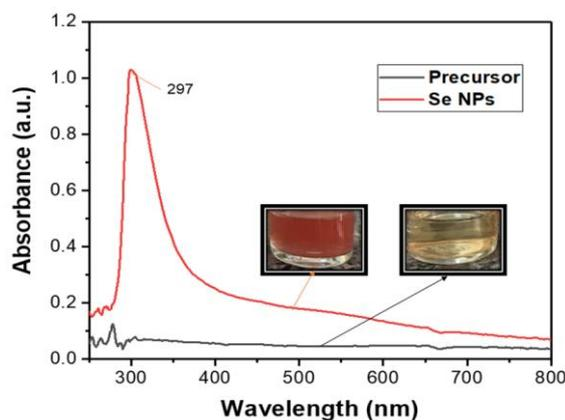
Figure 3. UV-vis absorption spectrum of the product.
