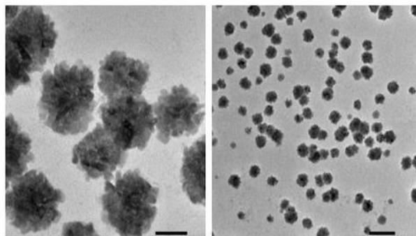
Figure 8. TEM image of as-synthesized nanoselenium.
