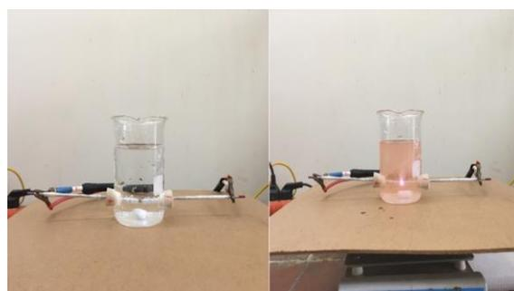
Figure 2. Synthesis process of nano selenium after 60 mins of reactions using distilled water and ethanol mixture as solvent.
